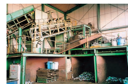
Automatic sorter Steel and aluminum cans are sorted by magnetic force
