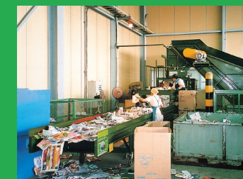
String-cutting machine and work for removing foreign matters manually
