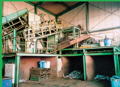
Automatic sorter Iron and aluminum cans are sorted by magnetic force.
