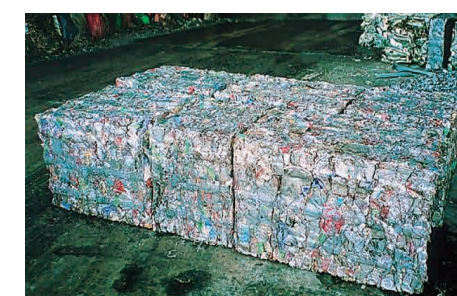
Pressed block Cans are compressed for easy carrying
