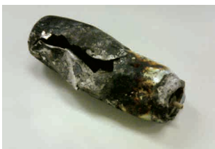
A spray can that ruptured and caught fire inside a garbage truck
